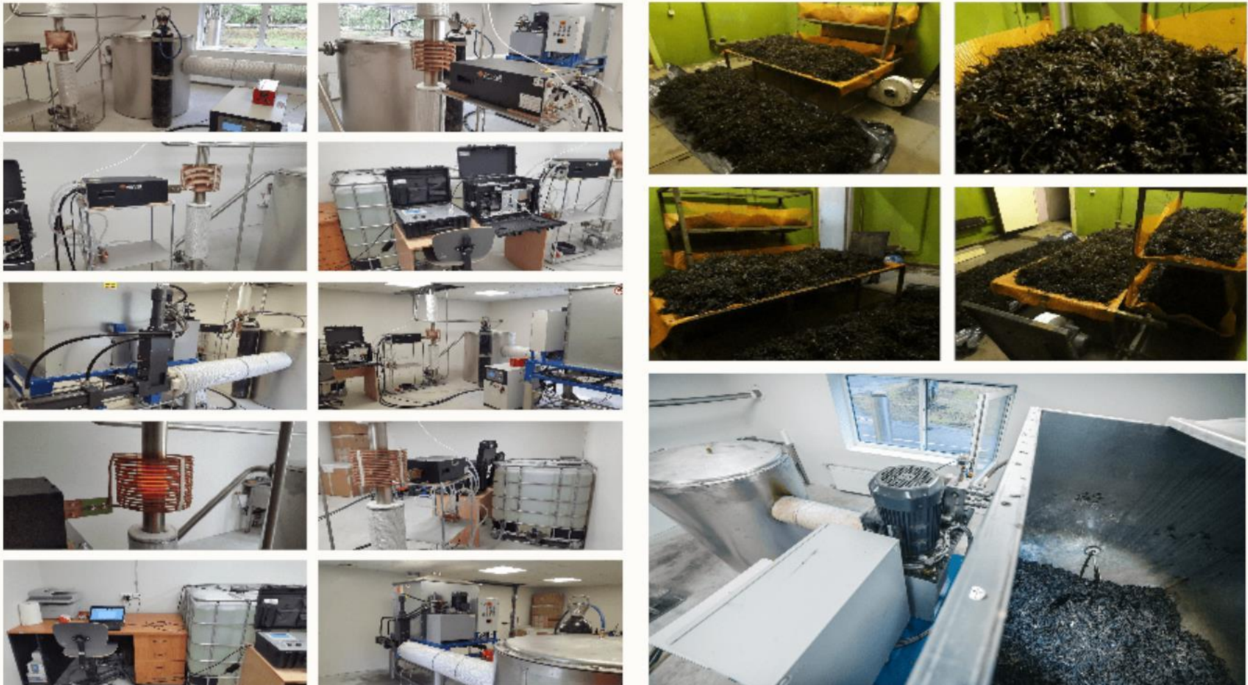
Left: Gasification unit with feeding system, pyrolysis chamber, gas cracking and gas measurement equipment. Right: Beach wrack drying and loading for gasification.
